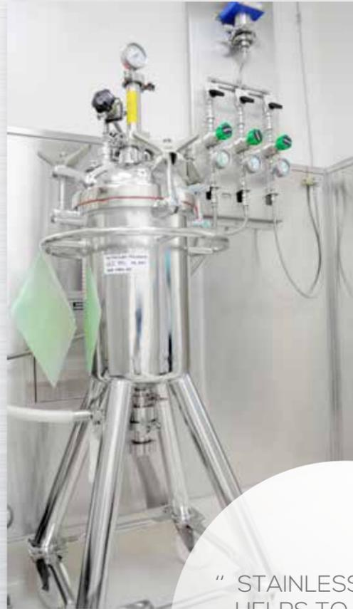
Stainless steel **does not react** with the chemical and biological substances used to produce pharmaceuticals. Its surface characteristics can be enhanced, e.g. by electropolishing, to minimise adhesion and optimize cleanability to the exacting standards of pharmaceutical and biochemical processes. Stainless steel helps to mass-produce medicine and make it widely available.
