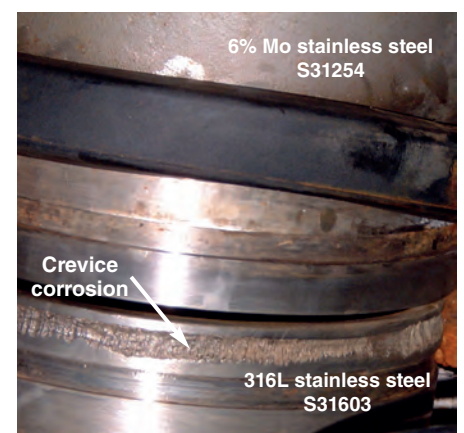
Figure 1: High-pressure couplings from a 40,000 m 3 /day seawater RO plant in the mediterranean basin. The 6% molybdenum coupling was in service for 7 years compared to only 6 months for the 316L coupling. © Piedmont Pacific Corp
