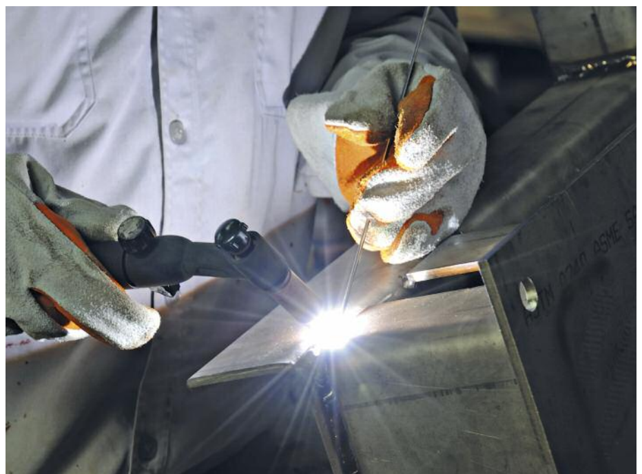
人工GTA(TIG)焊。© iStock.com/Lekyum
