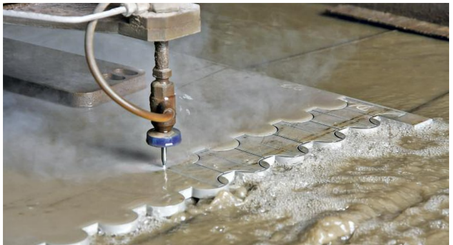
水射流切割不锈钢板。© Lubos Chlubny/Shutterstock.com
