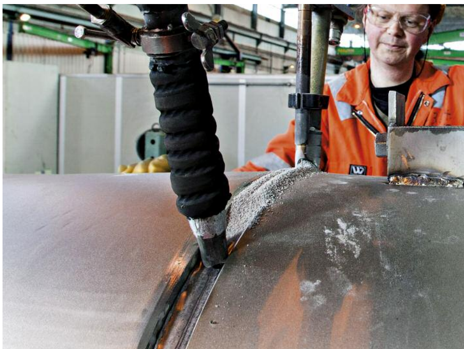
埋弧焊。© ESAB Welding & Cutting
