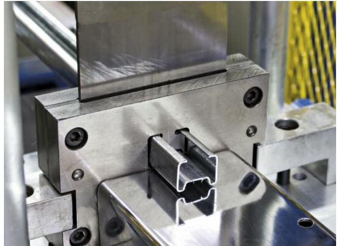
辊轧成形机加工的槽形不锈钢。© Warut Sintapanon/Dreamstime.com
