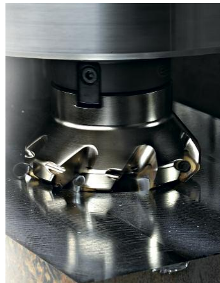
用硬质合金刀具对奥氏体不锈钢进行平面铣削。© Seco Tools
