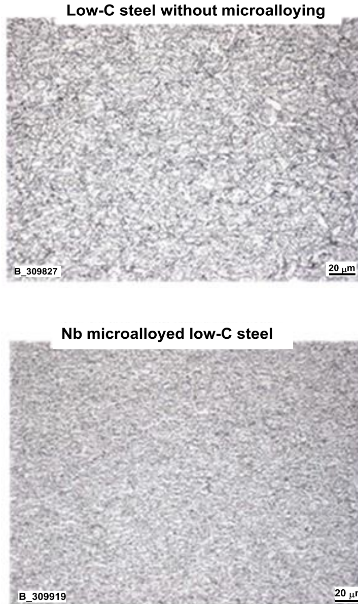
Figure 6. Effect of Nb microalloying on bainitic microstructure of low-C DP steel after coiling at 500 °C.
