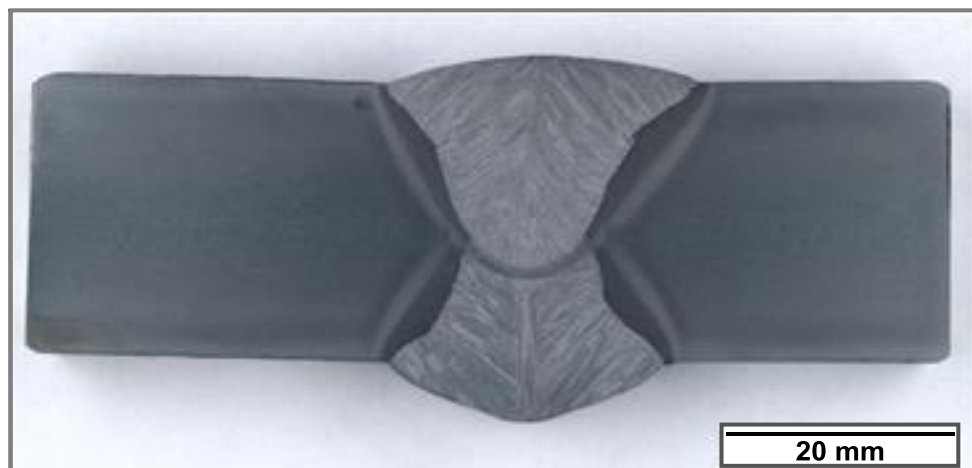
Figure 9. Cross section of SA weld, Nb content 0.022%.
