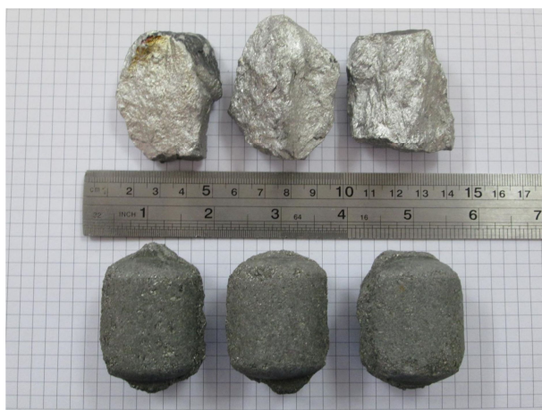
Figure 2. FeNb lump (top) and briquette (bottom).
