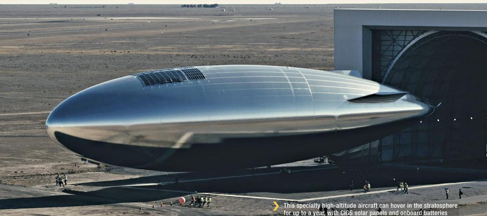
➤ This specialty high-altitude aircraft can hover in the stratosphere for up to a year, with CIGS solar panels and onboard batteries powering its observation and communications systems. © Sceye
