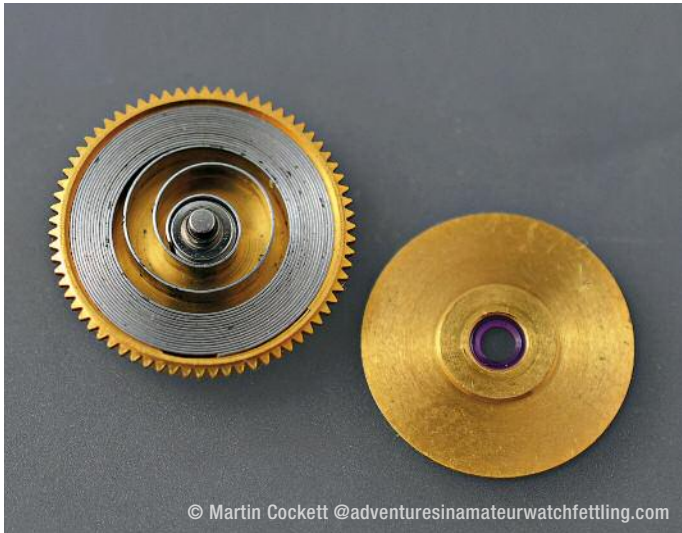
➤ Mainspring in the barrel (left) and unleashed for cleaning (right). As mainsprings are wound with such force, they must be removed by a special tool to not injure the watchmaker!
