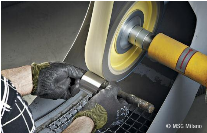
➤ Hand polishing is a step in the production of this stainless steel fitting.
