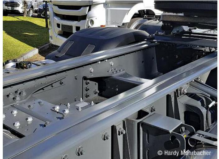
➤ Using a stronger steel means that the cross section of the trailer beams can be reduced, making the trailer lighter.
