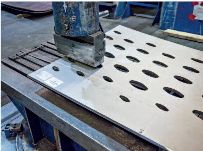
The lasered stainless steel sheets are formed three dimensionally on a heavy press (left). Afterwards these sheets are welded together into four quarters. The 'folded' edges that reinforce the lightweight shell construction are actually attached by welding. © Wilfried Dechau
