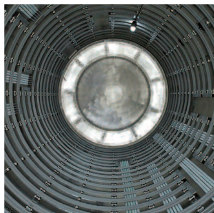
The inside of a typical HIP furnace. Molybdenum is used for the heating elements encircling the 'hot zone', the structure that supports the elements, 'furniture' that supports the furnace load, and thermal shielding that surrounds the hot zone. © Quintus Technologies
