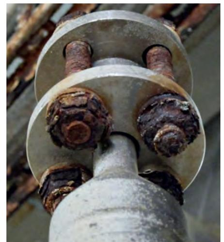
Hot dip galvanized bolts suffer from corrosion when exposed to the severe marine environment on a platform. © Statoil
