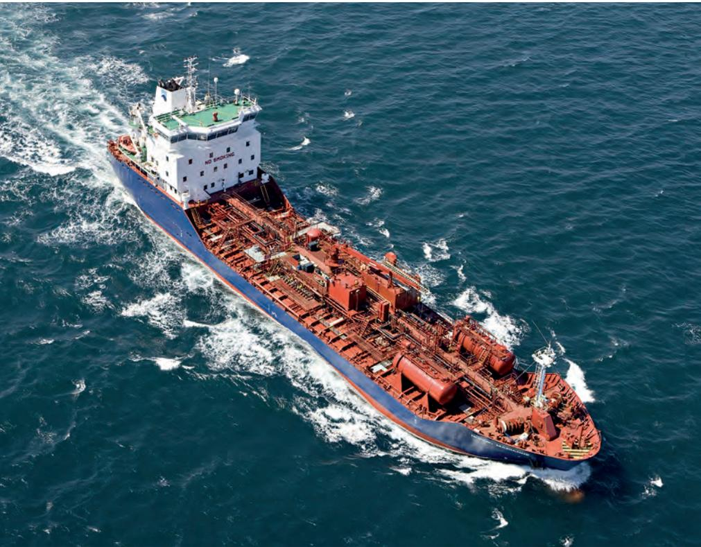
The topside of a chemical tank ship is busy with a myriad of pipes and valves. © Nordic Tankers
