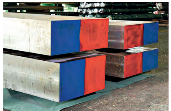
The mold is machined out of a block of mold steel produced by a specialty steel producer. © Alloy Tool Steel, Inc.
