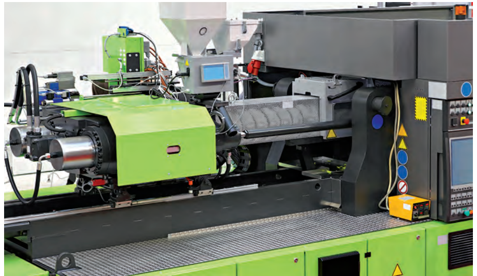
Injection-molding machines come in a range of sizes and production speeds, but all have the basic features of a resin delivery and molding system. © iStockphoto/Baloncici
