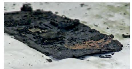
Resin and fiberglass crumble and turn into ashes while precious metal components remain intact and can be sorted. © CNRS
