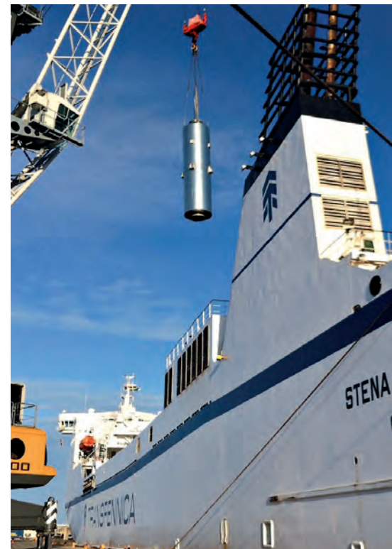
A marine FGD scrubber vessel being retrofitted to a cargo ship. © CR Ocean Engineering
