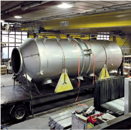
The scrubber vessel of a marine flue gas desulfurisation (FGD) unit ready to be shipped. © CR Ocean Engineering
