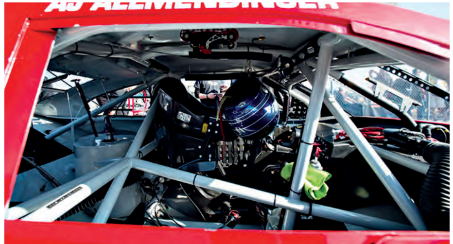
The roll cage inside a NASCAR vehicle is designed to protect the driver in case of an accident. © Sean Klingenhoefer
