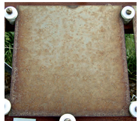
316L grade (left) and 409 grade (right) plates after 17 years exposure at Sellafield. © NNL
