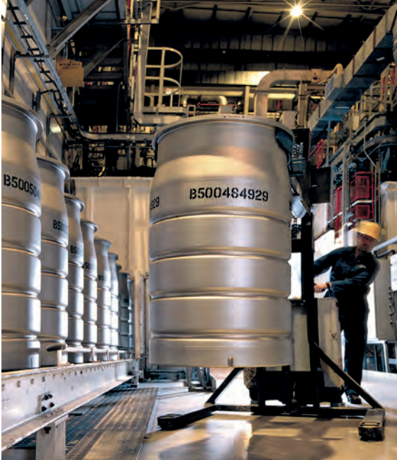
Intermediate level waste drums at Sellafield made from Type 316L stainless steel. The drums are filled with waste and stored in stacks (one stack of ten drums under each white square with the yellow dot) in the Encapsulated Product Store at Sellafield, prior to final geological disposal. © Sellafield Ltd
