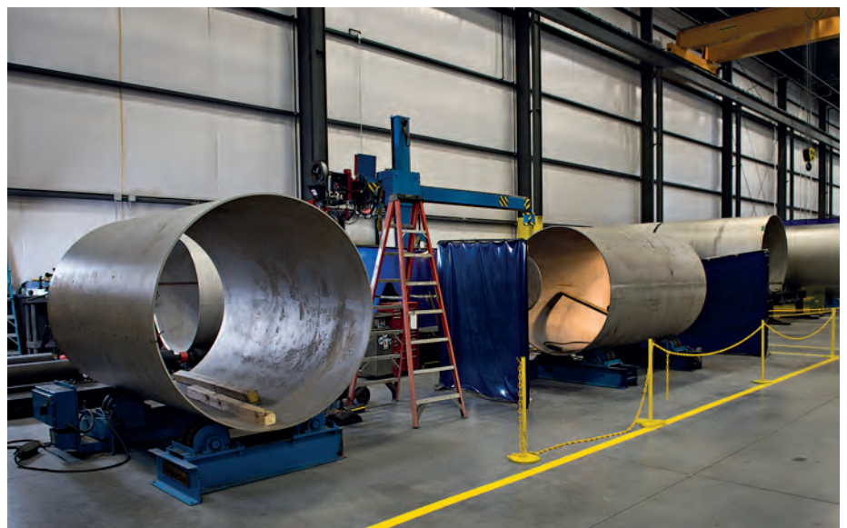
Duplex dry storage canisters being manufactured in North Carolina, U.S. © AREVA TN
