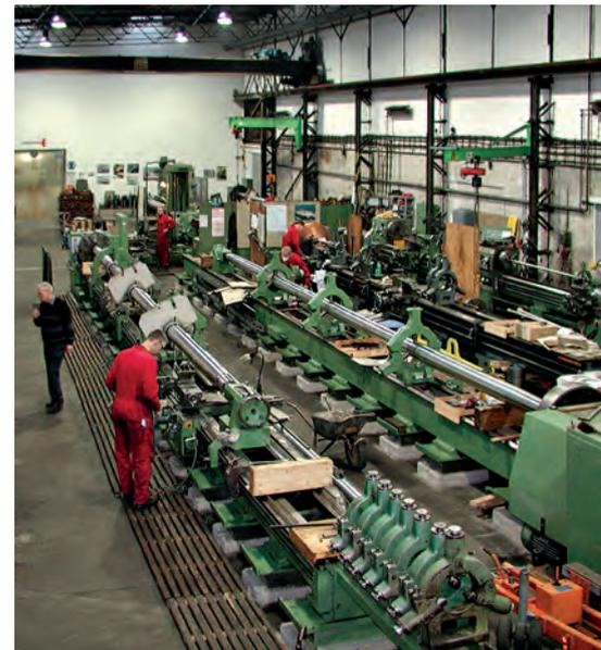
The fabrication of boat shafts requires large, sophisticated machinery to maintain the tight tolerances necessary. © Schaffran Propeller + Service GmbH
