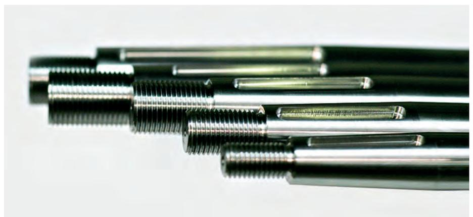
Boat shafts require precise machining of the taper where the propeller is attached.
