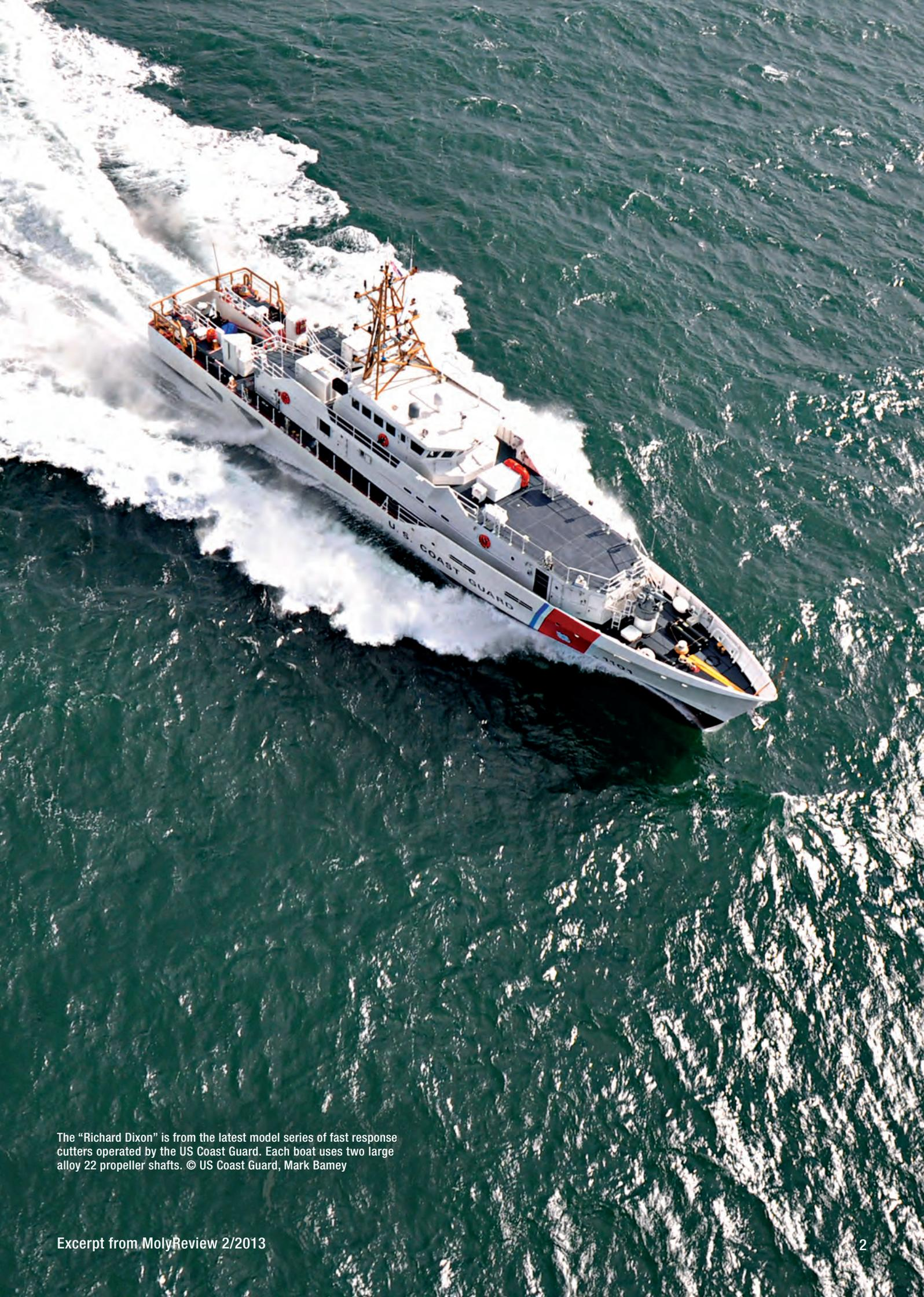
The "Richard Dixon" is from the latest model series of fast response cutters operated by the US Coast Guard. Each boat uses two large alloy 22 propeller shafts. © US Coast Guard, Mark Bamey
