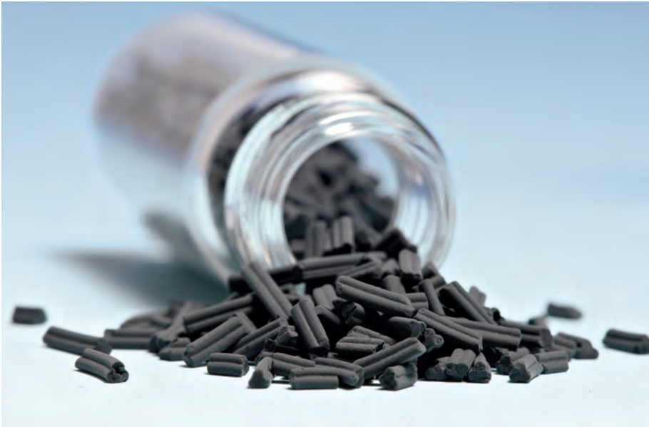
Molybdenum-containing catalysts dramatically reduce the sulfur content of oil-based fuels. © Haldor Topsøe
