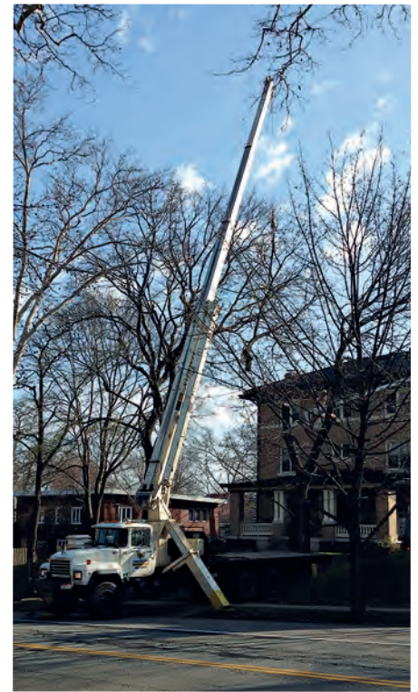
Truck cranes are highly versatile, and are seen in a wide variety of lighter lifting applications such as this tree extraction. © Robert Bukk
