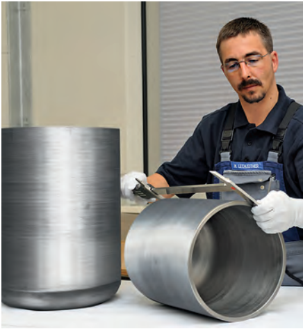
Molybdenum metal crucibles for sapphire production. © Plansee
