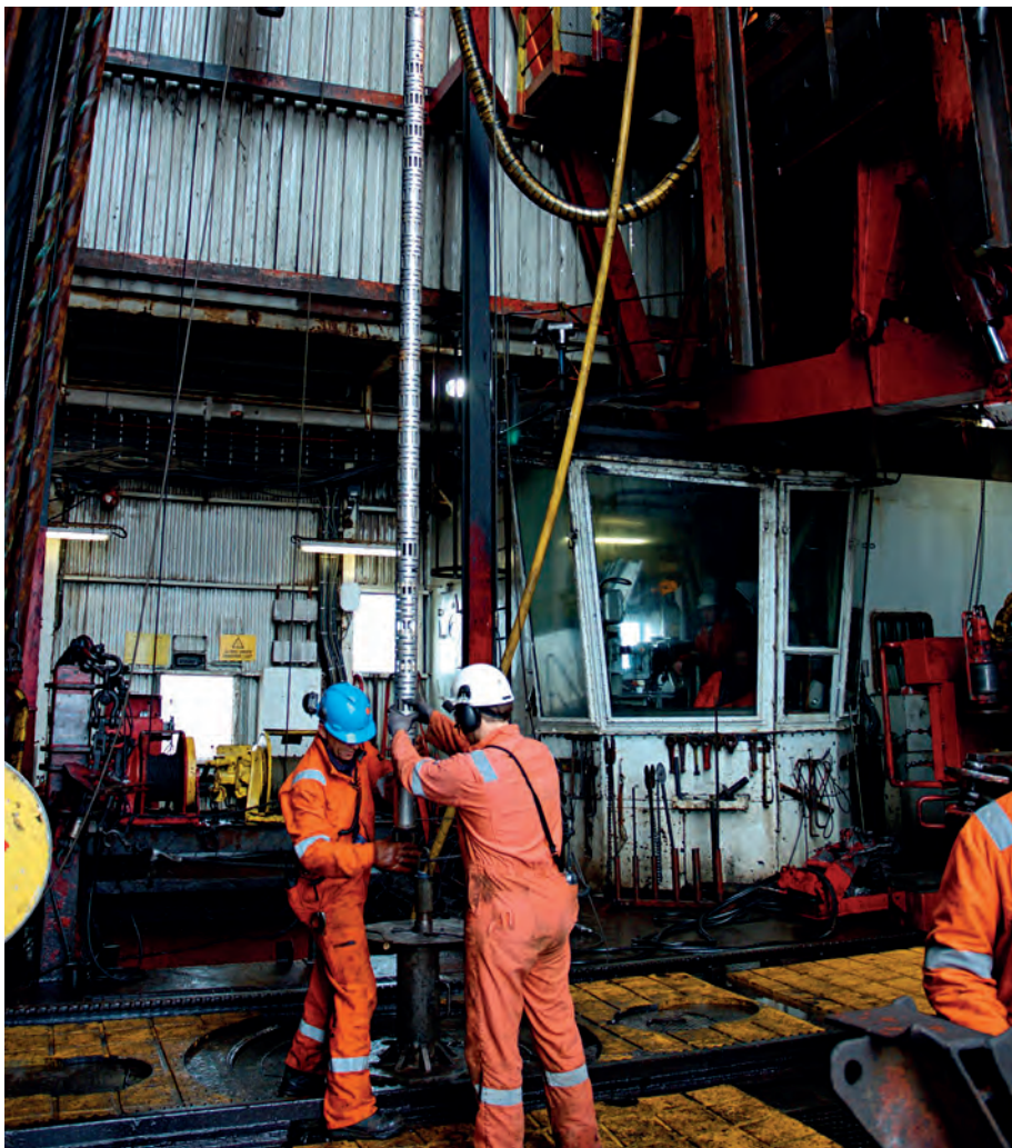
The crew is preparing to lower wireline equipment downhole for logging on an offshore oil rig. © Ingvar Tjostheim/shutterstock.com
