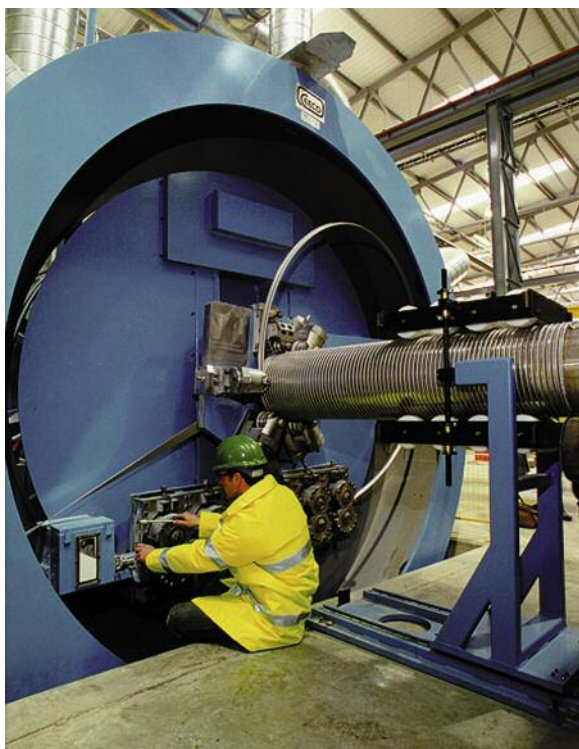
Figures 3 and 4: Strip forming into pipe with cross profile of s-interlock.
