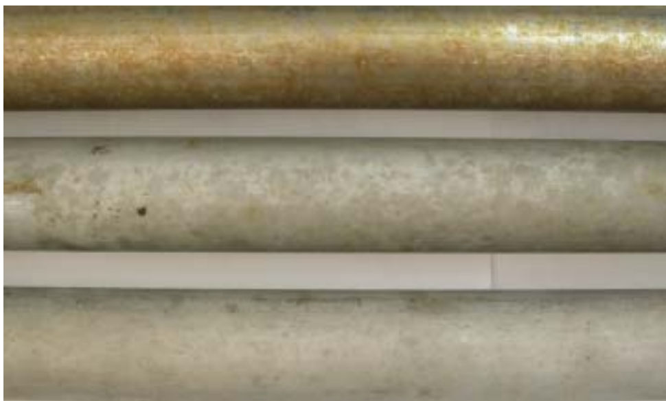
Figure 4. The pickled tube samples after fifteen months exposure in the splash zone displayed uniform, red staining on the 316L (top), light, localized staining on the S32003 (middle), and very limited stain spots on the 2205 (bottom) tube.
