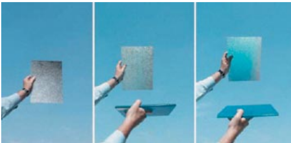
Placement of the blue panels was determined by varying the panel angle relative to the spandrel to obtain optimal reflection onto the spandrel panels.
