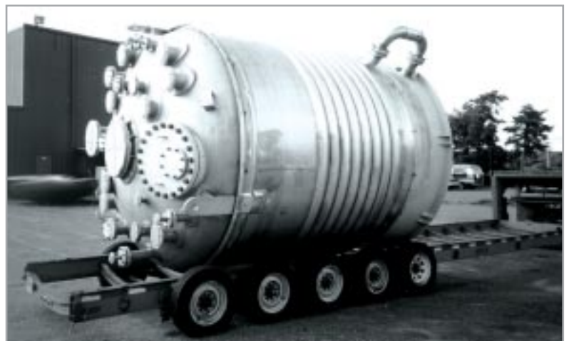
Figure 1: Process vessel constructed in 6% molybdenum stainless steel.
