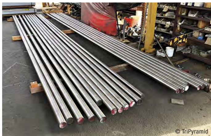
▶ 车间内待安装的2205双相不锈钢拉杆
