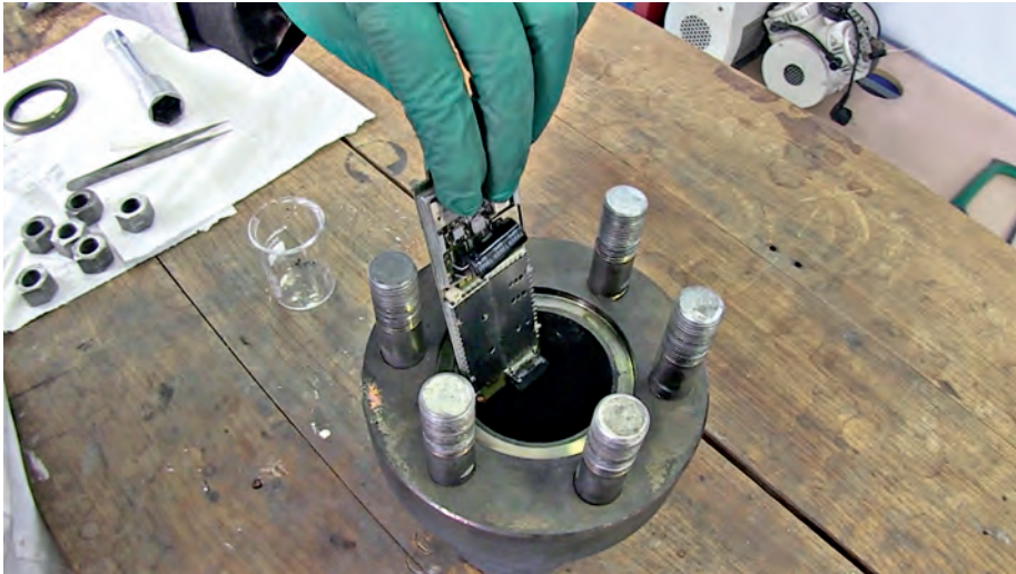
The recipe: plunge the board into supercritical water and cook it for about 30 minutes. © CNRS
