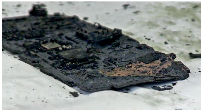
Resin and fiberglass crumble and turn into ashes while precious metal components remain intact and can be sorted. © CNRS
