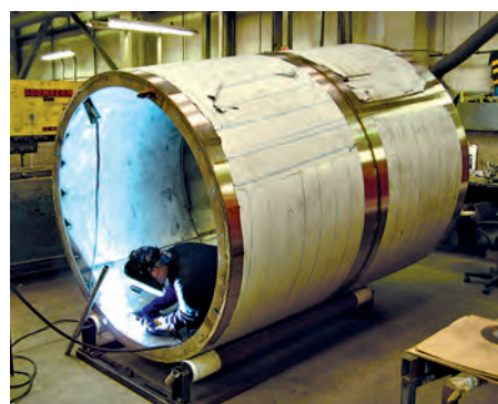
Fabricating a shell section of the Roancarrigmore lighthouse tower. © Commissioners of Irish Lights
