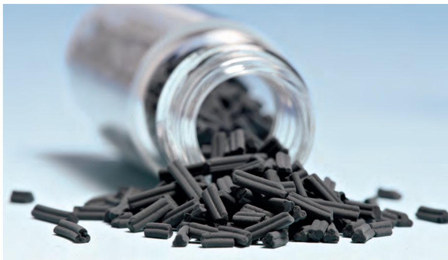
Molybdenum-containing catalysts dramatically reduce the sulfur content of oil-based fuels. © Haldor Topsøe
