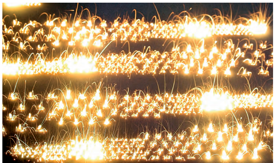
Lasers fuse metal powder during 3D printing. © www.siemens.com/press
