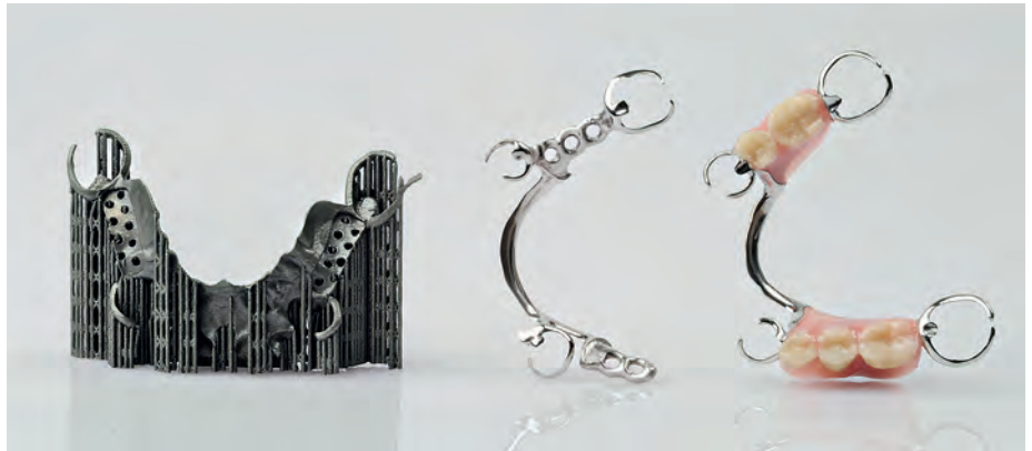
...and to make the metal part of very intricate partial dentures. The production stages from left to right: partial denture directly after 3D printing on its support structure, support structure removed and polished and after completion. © EOS
