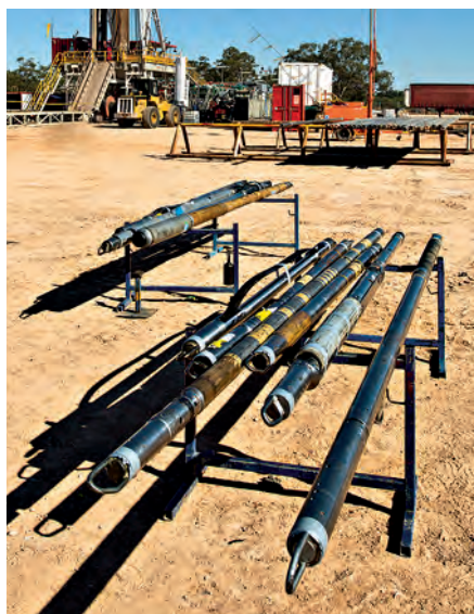
Logging tools that are ready to be lowered into the well with wireline. © Downunderphoto–Fotolia.com
