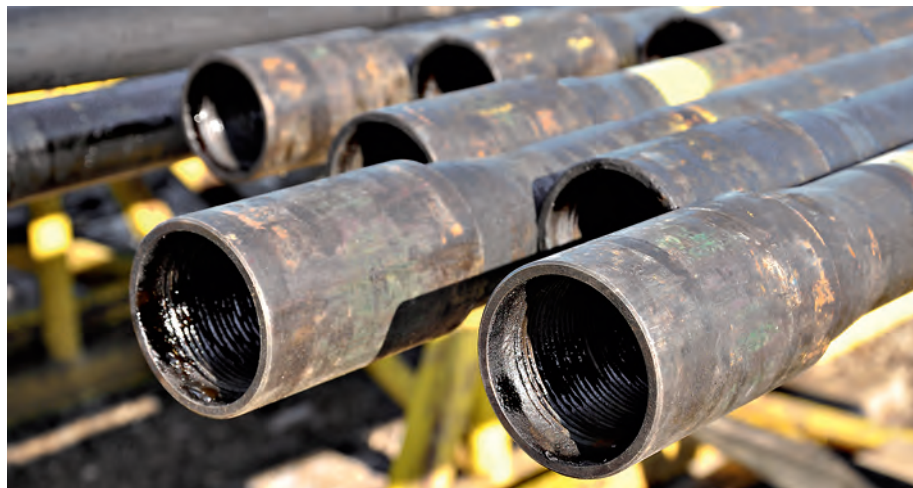
Drill pipes of 9.4 meters in length are attached to each other with threaded connections to build up a kilometer long drill string. © istockphoto.com/wpohldesign
