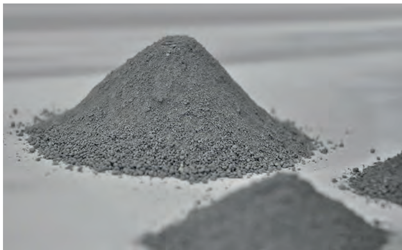
Molybdenum trioxide powder is used today by steel companies when adding molybdenum to stainless and alloy steels in the melt shop. Photo: Molymet
