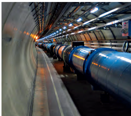
The LHC tunnel showing the line of blue superconducting magnets which are the major components of the LHC. The curve of the tunnel can be seen in the distance. Photo: LHC
