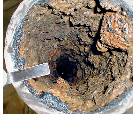
Inside diameter of carbon steel piping showing the fouling/bio-fouling typical of the problems encountered in service water piping.
