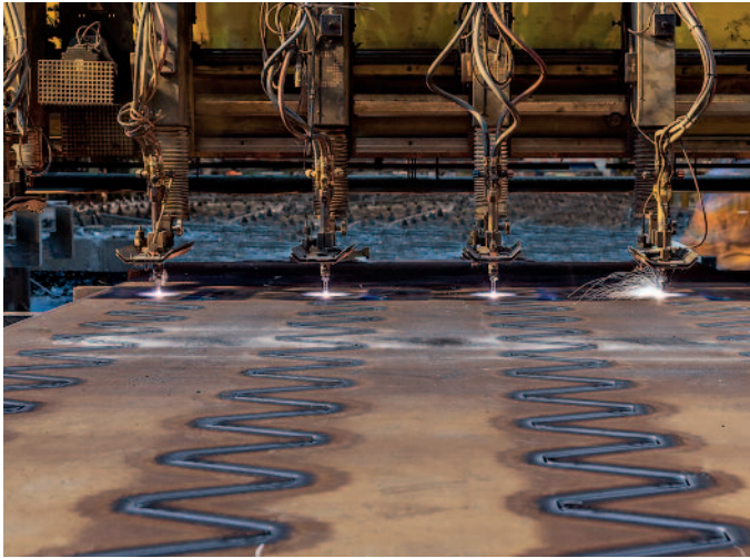
The shape of gear racks is produced by flame cutting heavy plates. © Dillinger
