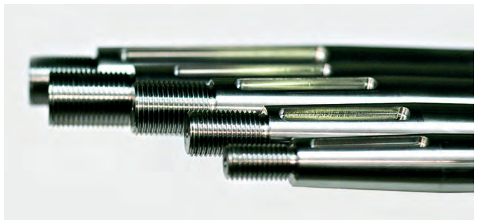
Boat shafts require precise machining of the taper where the propeller is attached. © Clements Engineering
