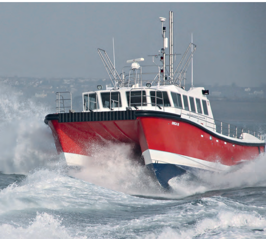
This work boat has two 90 millimeter diameter 2205 duplex stainless steel shafts. It is designed to bring crews to offshore wind farms. © Clements Engineering
