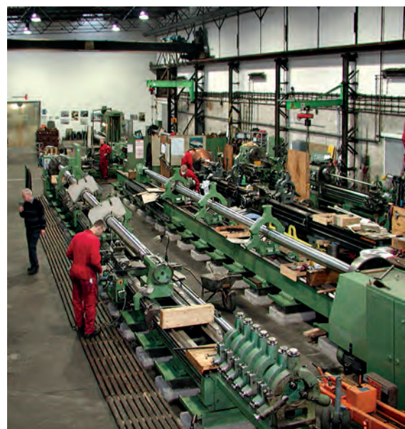
The fabrication of boat shafts requires large, sophisticated machinery to maintain the tight tolerances necessary. © Schaffran Propeller + Service GmbH
