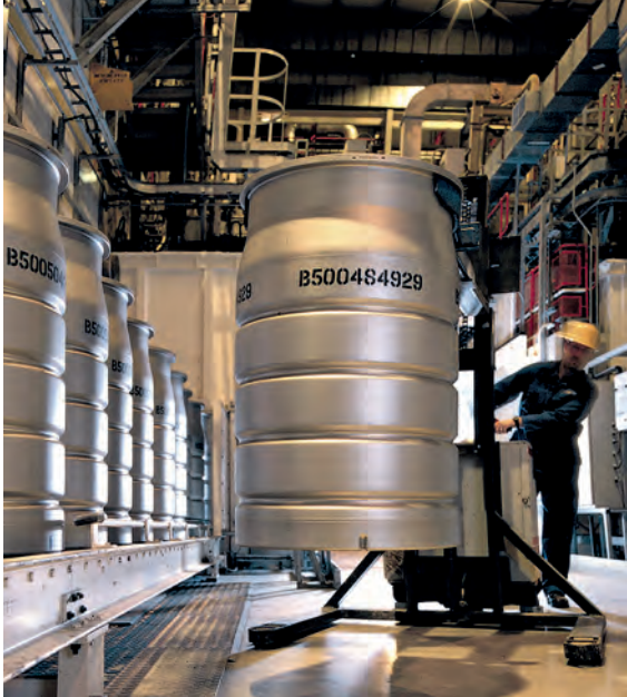
Intermediate level waste drums at Sellafield made from Type 316L stainless steel. The drums are filled with waste and stored in stacks (one stack of ten drums under each white square with the yellow dot) in the Encapsulated Product Store at Sellafield, prior to final geological disposal. © Sellafield Ltd
