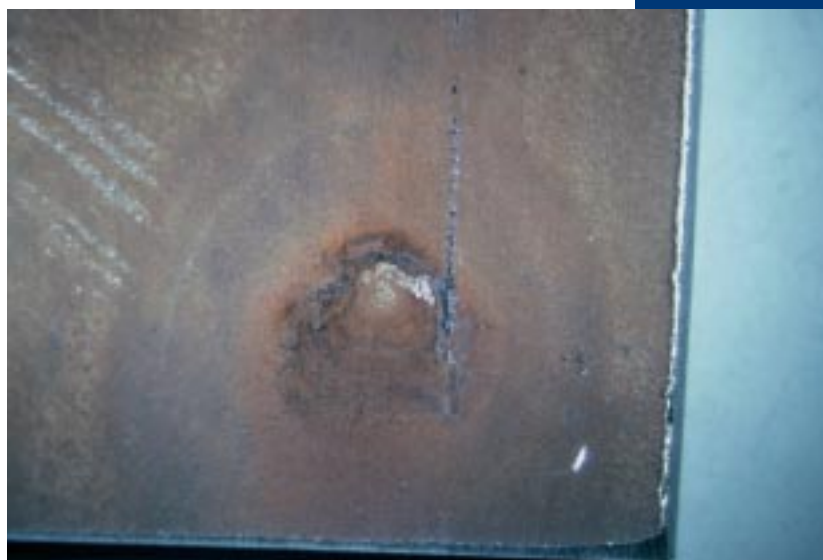
Fig 2: Close-up of the pitting corrosion.
