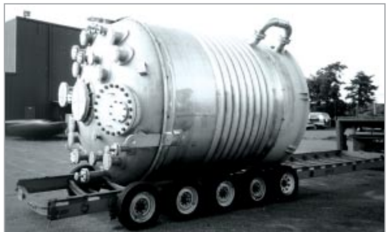
Figure 1: Process vessel constructed in 6% molybdenum stainless steel.
