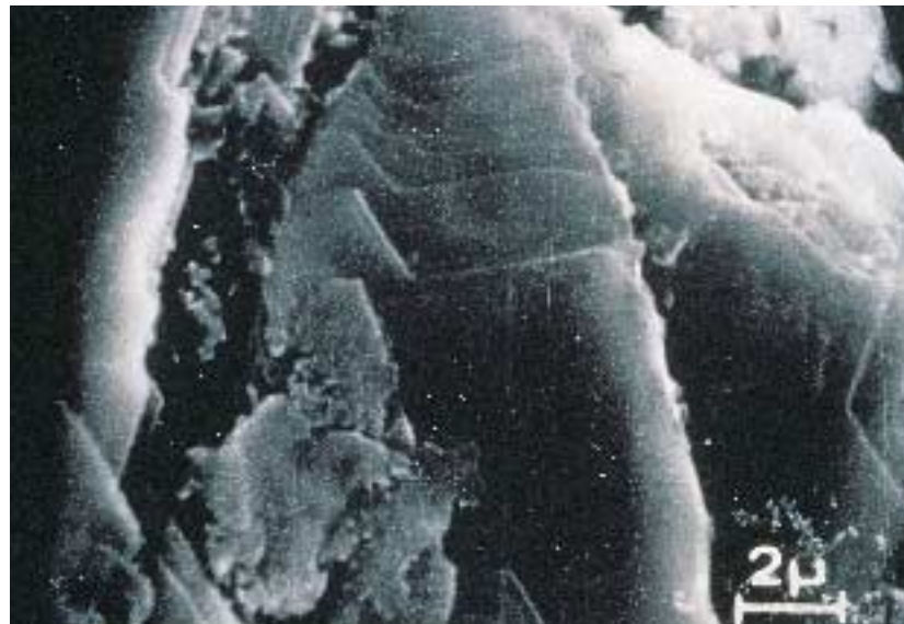
Cross-section of a molybdenum disulphide film showing the plate-like structure
