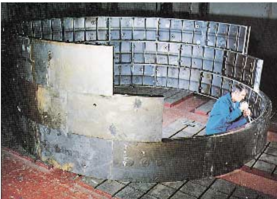
London Tube tunnel linings use highly alloyed super duplex stainless steel
