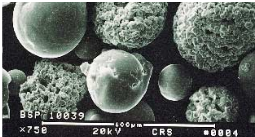
Spherical Agglomerates of Mo Powder (lacy appearance), with solid spheres of the Ni-Cr alloy binder for the Mo powder
