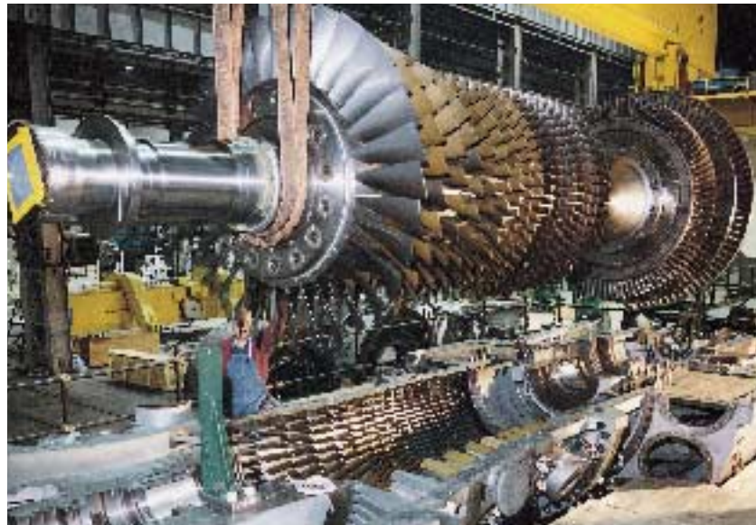
Rotor of a gas turbine, type FR 9001/E, 170 MW, with high Molybdenum-containing steel blades (Courtesy of Nuovo Pignone, Firenze)
