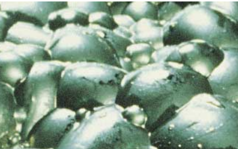
Molybdenite particles coat bubbles during flotation process
