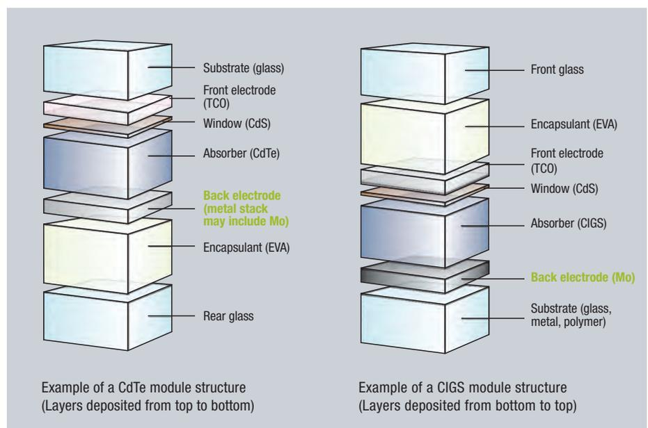
Figure 3: Schematics of the layered construction of thin film solar cells. Molybdenum plays a critical role as a preferred back electrode. Source: Prismark Partners, LLC
