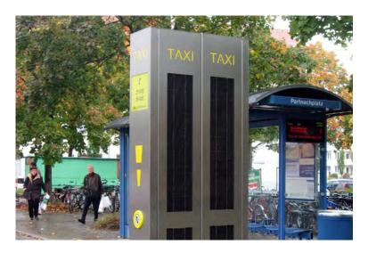
Thanks to an intelligent combination of battery and photovoltaic technology, the 176 taxi call points installed so far save around 100,000 kWh of electricity per year.
