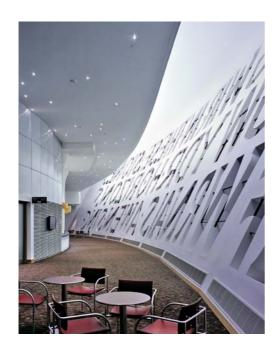
Moulded casings, inside and outside, make up the individual letters. A grid of flat steel, painted matt black, further strengthens the contours of the cut-out letters.
