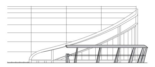
Both leaning pads and cable barriers are supported on inclined 'T' section stanchions made from matching 1.4401 stainless steels.
