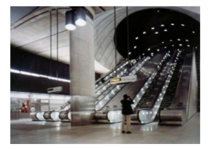
Foster and Partners used a simple palette of hardwearing constructional materials – unadorned concrete, glass, and stainless steels. This robust aesthetic is most pronounced at platform level, where satin finish stainless steel clads the oval-section columns in a critical damage-prone area.
