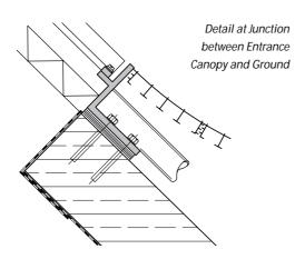
The stainless steel angle section 240 by 250 by 20 mm thick supports the structure through size M20 stainless steel bolts to BS EN 3506, and is curved to match the canopy profile. Satin finished 1.4432 (X2CrNiMo17-12-3) is used for the section, which connects to the louvre grilles above via anti-theft wheelnut fixings, and is concealed by a loose fill at ground level.
