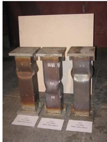
Figure 3. Tests on RHS with slender cross-sections
