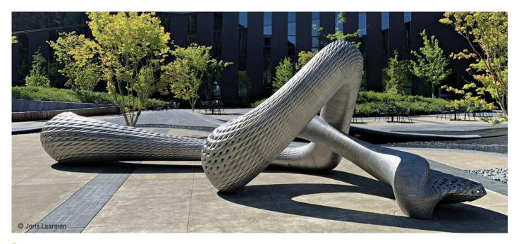
The elegant structure was shipped from Europe to the US West Coast in three parts and welded together on site. The surface undulations contribute to stiffening the structure.
