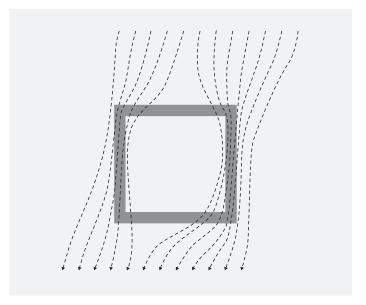
Mu-metal/aluminum walls deviate and block external magnetic fields around the magnetically shielded room. The space inside is practically free of a magnetic field.
