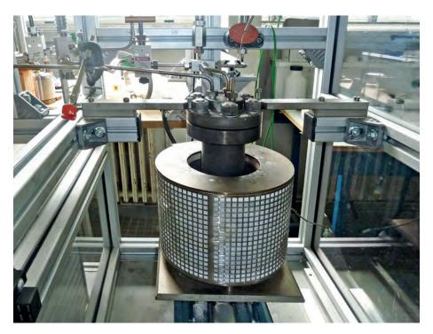
Prototype reactor for environmentally friendly electronic-waste treatment. © CNRS
