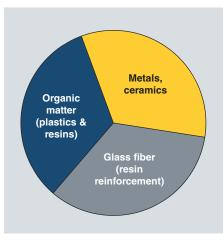
Electronic circuit boards: three main types of materials
