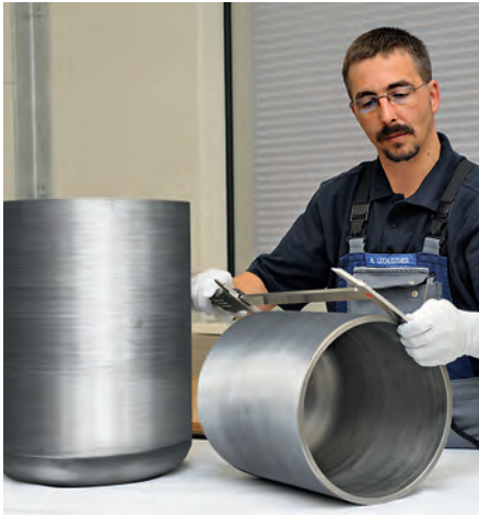
Molybdenum metal crucibles for sapphire production. © Plansee
