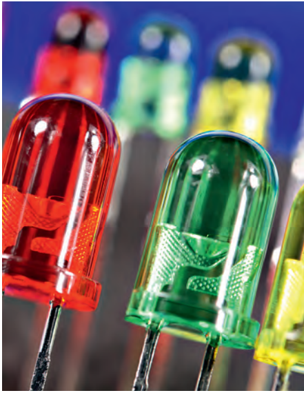
Individual LED lamps with epoxy dome dyed to indicate the color of light produced. © iStockphoto.com/JamersonG
