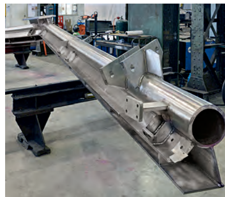
Straight or curved, duplex gutters are fitted with fixing "ears" and mounting plates. © Gérard Tordjman
