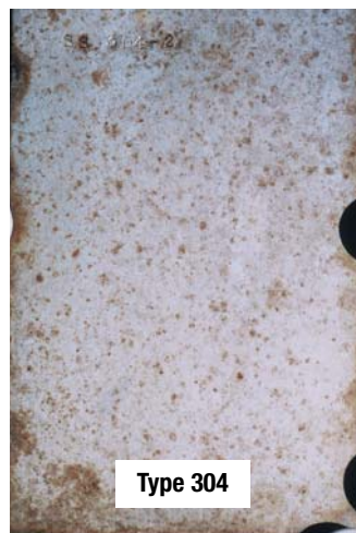
Figure C Kure Beach, North Carolina samples after 56 years. (Photo Courtesy of TMR Stainless)
